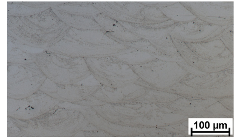
Microstructure without heat treatment (NHT)
