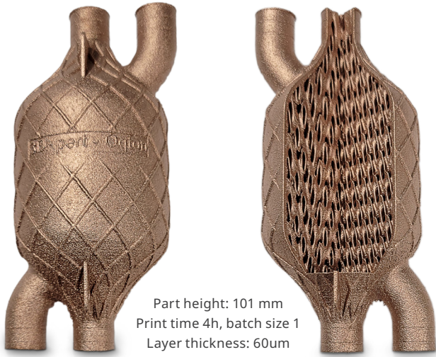
As-built surface quality with no post-finishing
