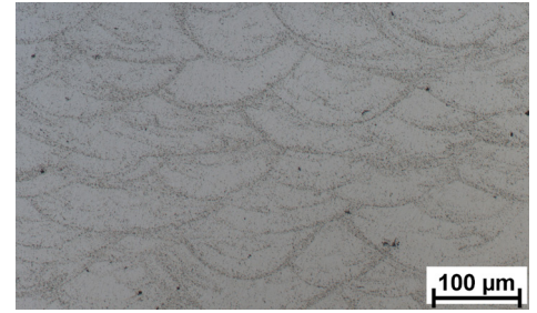
Microstructure after SR
